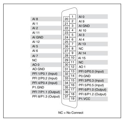
Figure A-2. NI 6233 Pinout
